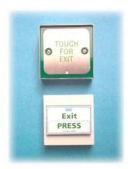
The switches shown opposite are both manually operated. The 'TOUCH FOR EXIT' switch is touch sensitive. The slightest contact of a finger or hand will activate the switch normally triggering the lock release to let callers in. This switch is suitable for persons with very little hand strength or coordination. These switches are normally use with hands free door entry systems or powered door openers.
